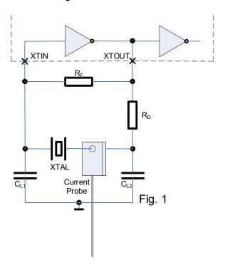
The crystal power level can be determined as follows:
